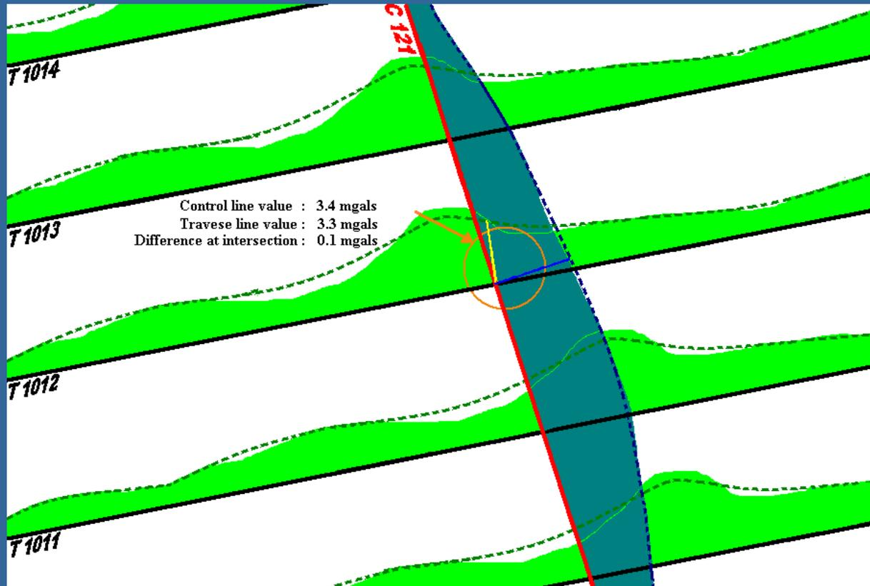
Line filtering will affect anomalies differently depending on line orientation.
