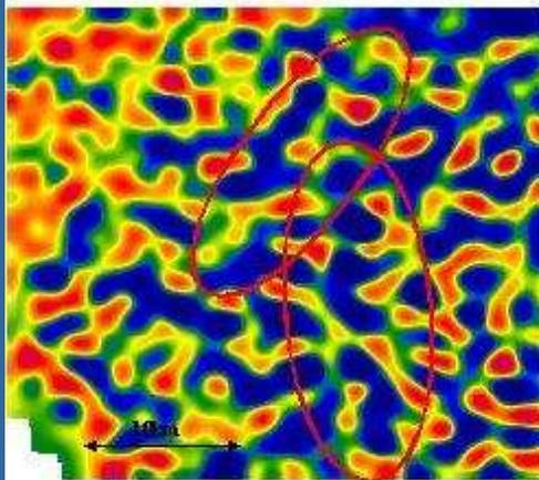
1<sup>st</sup> vertical derivative, ground Bouguer Gravity with sample lines
