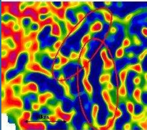
1<sup>st</sup> vertical derivative, ground Bouguer Gravity
