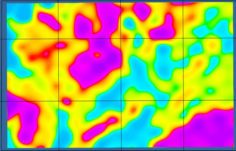
First vertical derivate of the AIRGrav grid with 10 km UTM lines
